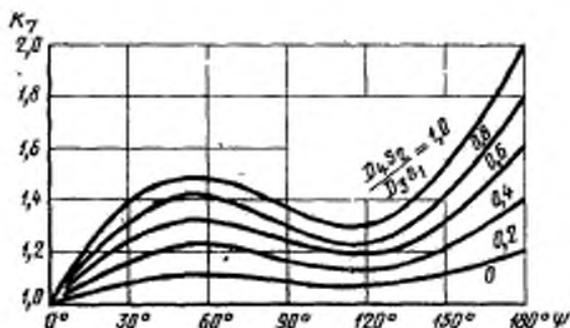
$$K_7 = 1 + \frac{D_4 s_2}{D_3 s_1} \left( \frac{\psi}{180^\circ} + \frac{\sin 2\psi}{\pi} \right) - \left( \frac{D_4 s_2}{D_3 s_1} \right)^2 \cdot \frac{2 \left( \frac{\sin \psi}{\pi} \right)^2}{1 + \frac{D_4 s_2}{D_3 s_1} \left( \frac{\psi}{180^\circ} \right)}$$
